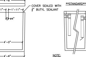
NOTE: INLET - SANITARY TEE OUTLET - SANITARY TEE W/ GAS FLAP SUPPLIED BY LAKELANDS INSTALLED BY CONTRACTOR
