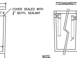
INLET - SANITARY TEE OUTLET - SANITARY TEE W/ GAS FLAP SUPPLIED BY LAKELANDS
